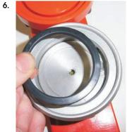
Ensure one Plastic Spacer Ring is in the Chrome Die. (Note-the 25mm machine does not use spacer rings)
