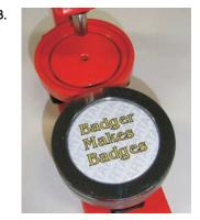
Place on top of this the metal Ring Die assembly from step 5, followed by the black Solid Die - flat side up.
