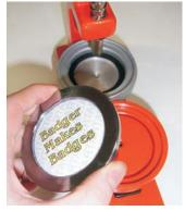
Remove the metal Ring Die WITH the shell+art+clear attached to it. DO NOT separate them.
