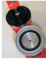
Put the Solid Die on top, flat side down, rotate the assembly under the pressing pin and press handle down firmly.
