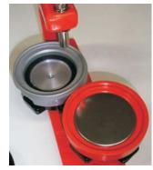
Using supplied circle cutter (not shown), trim artwork by pressing firmly on the knob and rotating handle only once. Fit the metal shell to the Orange Die.
